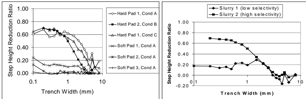
Figure 5 Metal Thickness Difference vs. Trench width for different pad-process combinations
