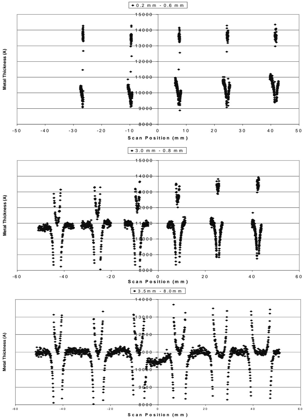
Figure 4. Insite 300 Metal Thickness Scans across the features of the Test Vehicles
