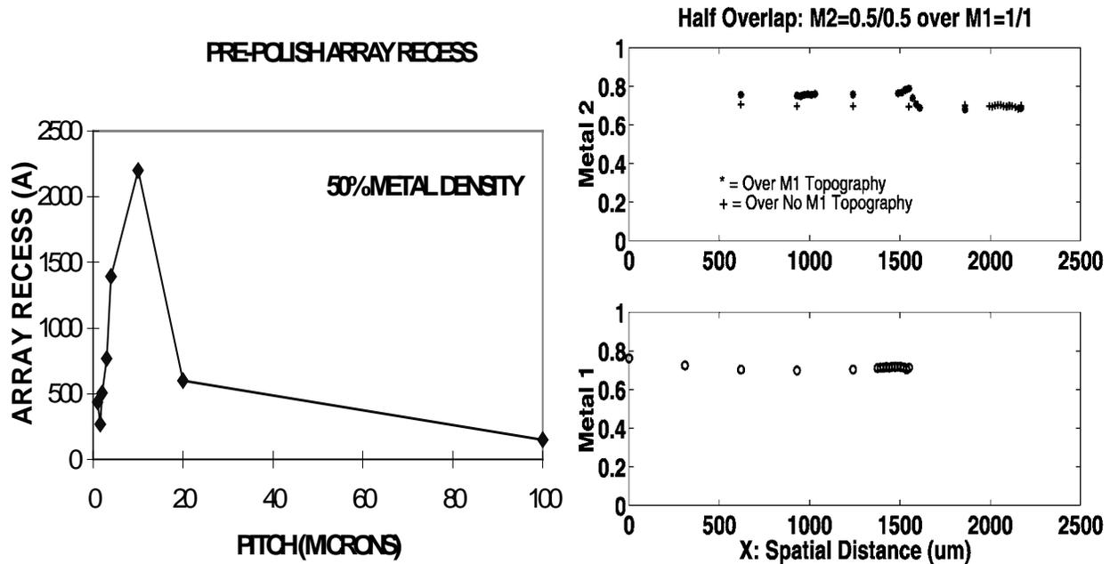
Figure 1 ‘Array-Scale Recess’ resulting from a copper electroplate process over a 50% metal density, 2500µm x 2500µm array as a function of pitch.
