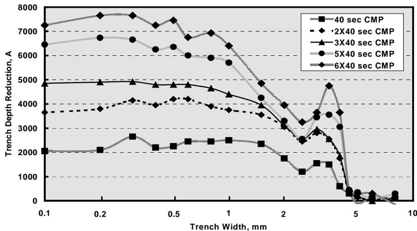
Figure 3 Trench Depth Reduction vs. Trench Width for equal time polish increments
