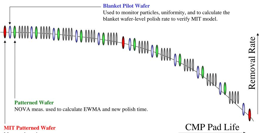
Measured ex-situ. Used to study the planarization length over the life of a CMP pad..
