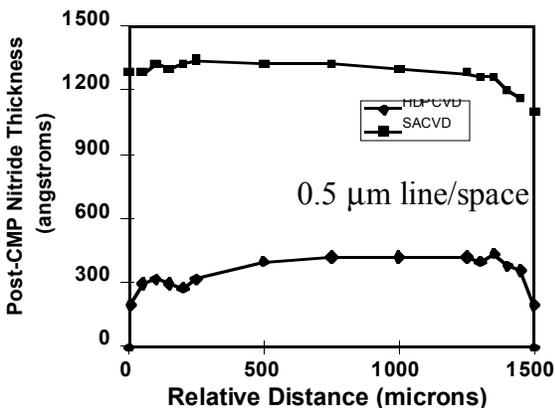
Figure 8. Different planarization behavior between HDPCVD and SACVD filled STI
