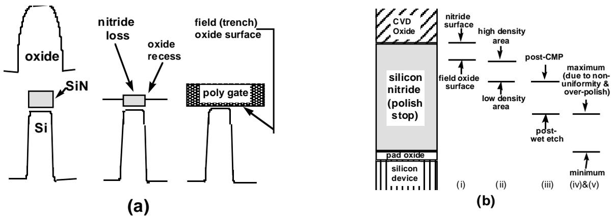
Figure 1. (a) Schematics of three intermediate STI structures: post-trench fill, post-CMP, and post-gate deposition; (b) key factors which consume available STI CMP budget
