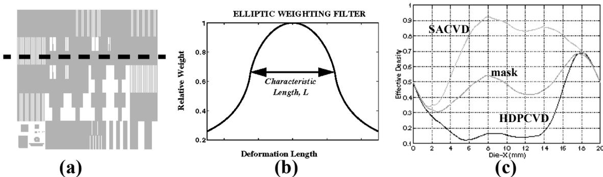
Figure 3. (a) STI CMP test mask, (b) elliptic weighting filter for effective pattern density calculation, (c) pattern density across the marked line in (a) for the mask and for SACVD and HDPCVD oxide
