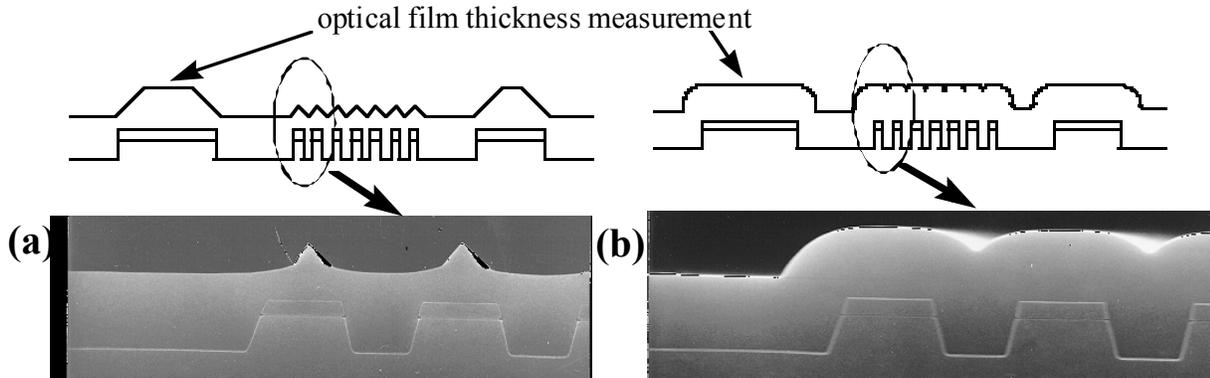
Figure 2. Oxide deposition profile over 1 μm line/space structure, (a) HDPCVD, (b) Giga-fill SACVD
