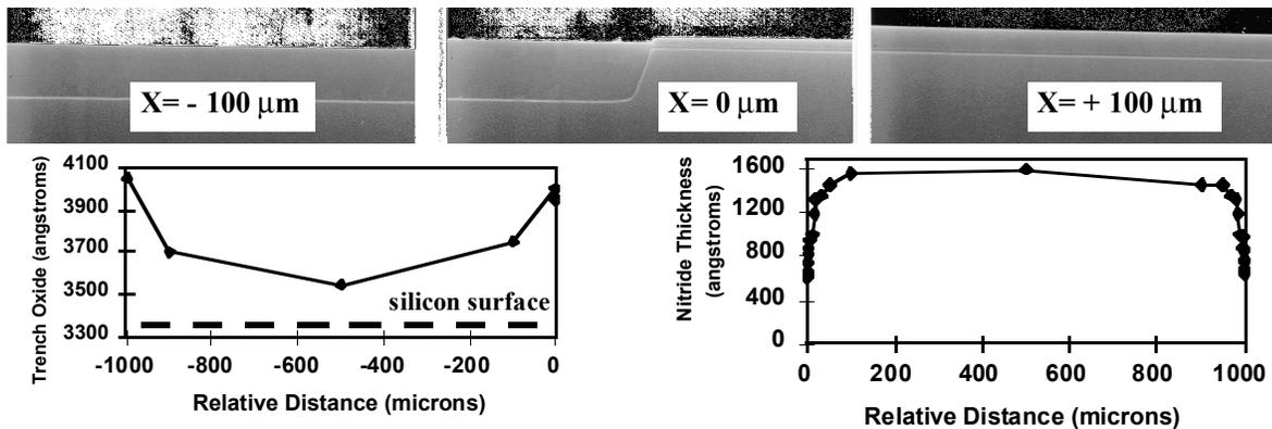
Figure 7. Trench oxide dishing and active nitride erosion across 1 mm wide trench and active feature
