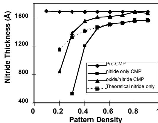
Figure 9. Selectivity degradation at lower pattern density region
