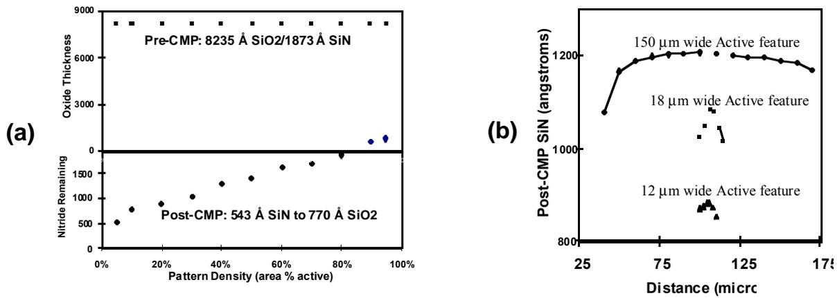
Figure 4. Post-CMP nitride thickness as function of (a) pattern density, (b) active feature size
